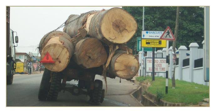
Figure 8: A timber truck with burst tyre and with logs almost falling off. Source: MadinGhana's blog.
