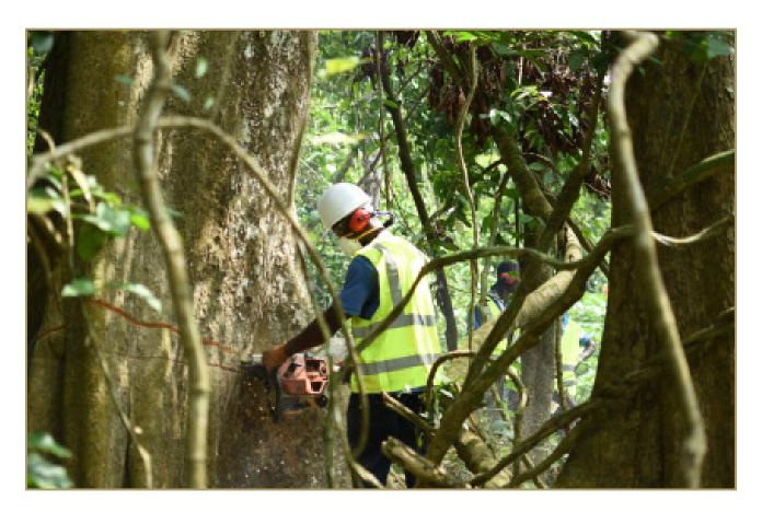
Figure 5: A chainsaw operator wearing appropriate PPEs. Source: NDF Training Team
